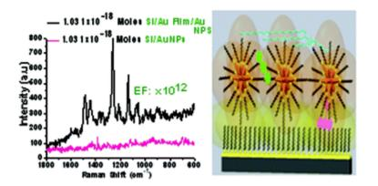
Graphical abstract: SERS substrates fabricated with star-like gold nanoparticles for zeptomole detection of analytes
